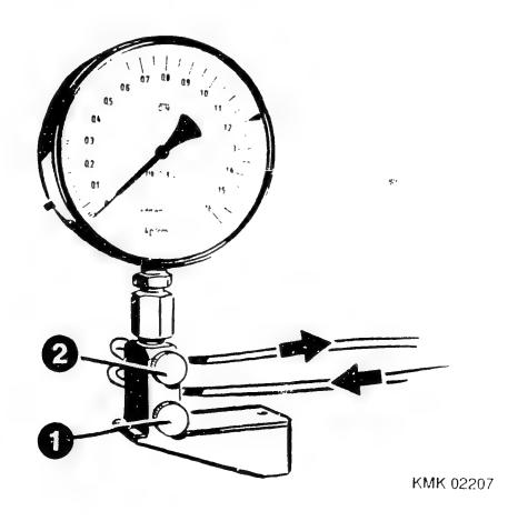
CHECKING MANIFOLD—PRESSURE COMPENSATOR (LDA)
